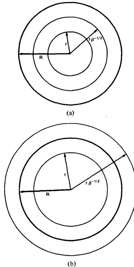
Fig. 4. (a) Case 1. Probability of no interfering traffic for  $\beta^{-1/2}r < R$ . (b) Case 2. Probability of no interfering traffic for  $\beta^{-1/2}r \geq R$ .
