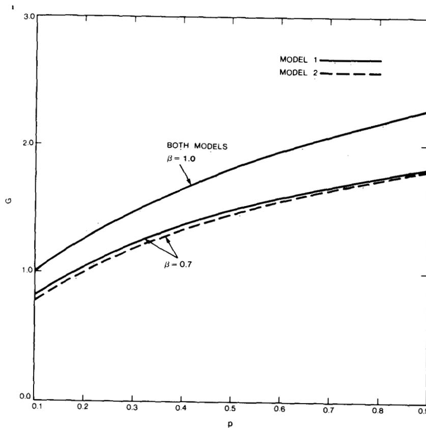
Fig. 9.  $G = Np$  as a function of  $p$  for optimal  $N$  and  $p$ , and  $\beta = 0.7$  and  $1.0$ .
